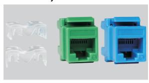
Delton Category 6 keystone jacks are RJ45 8P 8C 50U jacks suitable for 22-26 AWG stranded and solid wire, compatible with both 110 & Krone punch down tool. They are capable of retermination. They are available in universal labels color coded for T568A and T568B wiring schemes and fit in high density keystone patch panel. It complies with ANSI/TIA/EIA 568 C.2 standard and ROHs.
